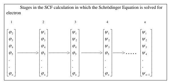
Consider electr. 1 and use a set of approx. WFs  $\varphi_2$  to  $\varphi_n$  to describe the remaining electrons. Solve the S.E. for electr. 1 getting  $\psi_I$
